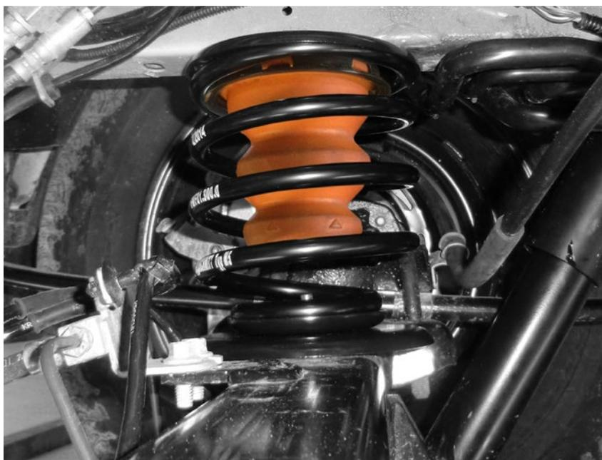
Leaf springs or torsion bars come standard on the rear axle of most transporter vans. As manufacturers do not primarily design their chassis with the intention of it being used as a motorhome or commercial vehicle later, the original springs often end up overloaded. Due to the high
